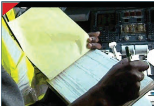
Figure 14-3. AMT documenting repair work.
