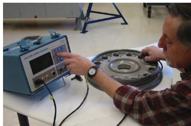
Figure 8-5. Eddy current inspection of wheel half.
