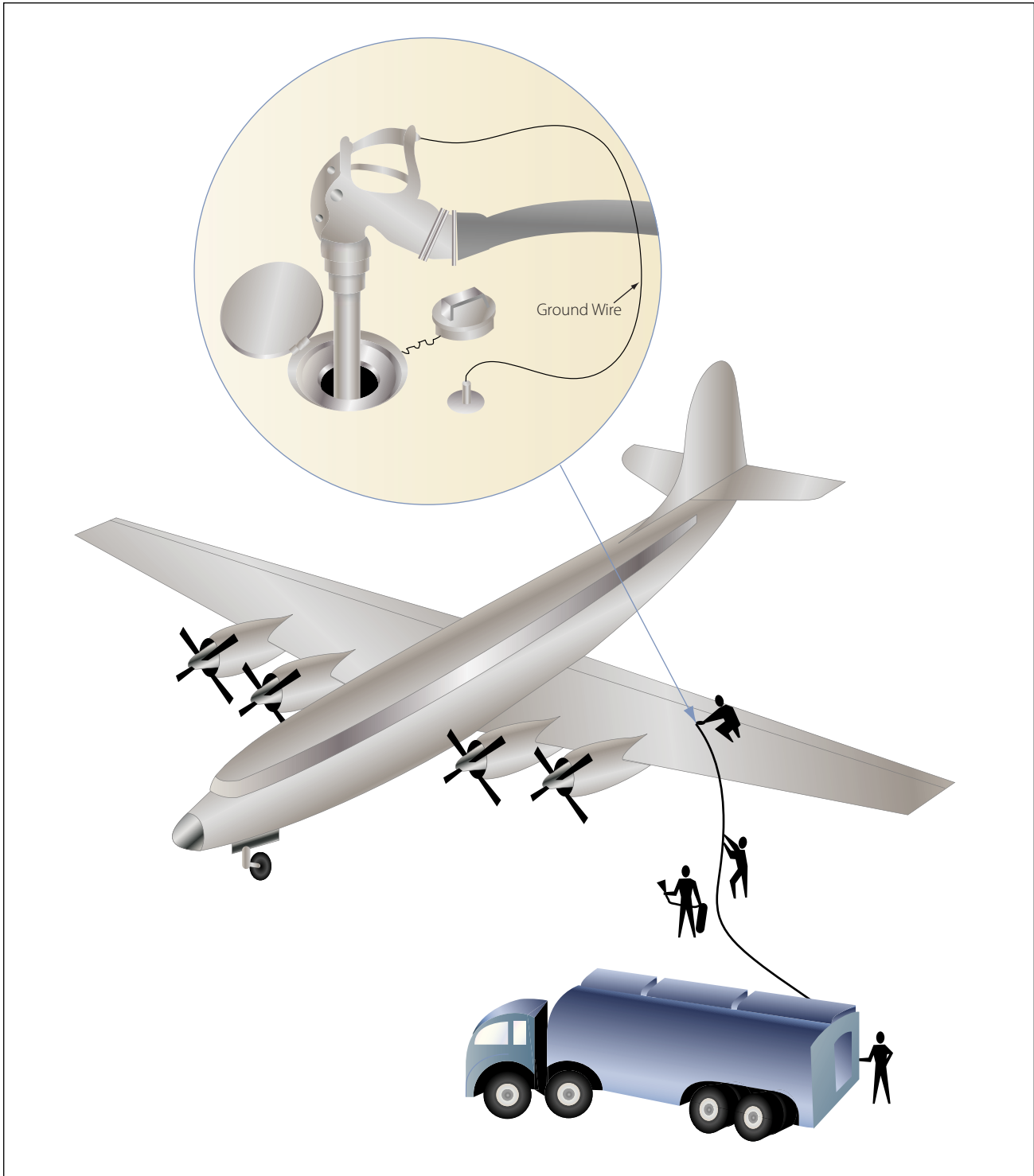
Figure 11-31. Refueling an aircraft by the over-the-wing method.
