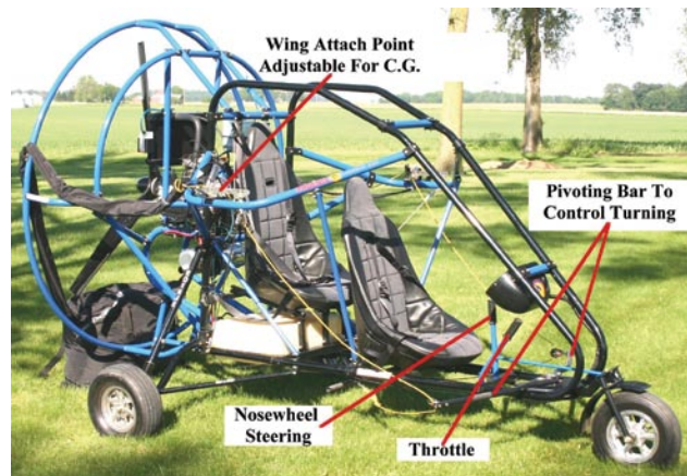
Figure 4-39. Powered parachute structure with wing attach points.
