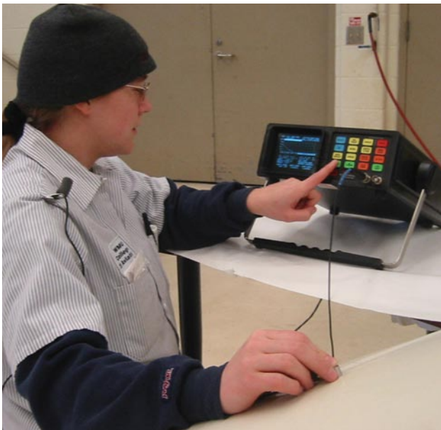
Figure 8-12. Ultrasonic inspection of a composite structure.
