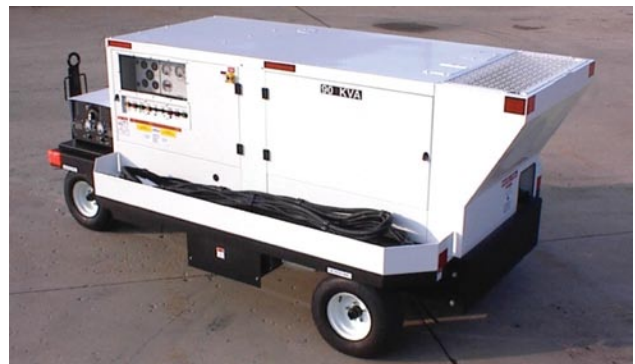
Figure 11-27. A mobile electrical power unit.
